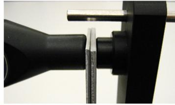
Adjust the distance to approx. 5 mm. (Use e.g. 2 + 3 mm aluminium absorbers.)
