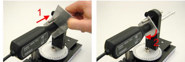
Placing absorber plates on the rod
