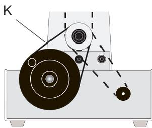
If you want to drive the belt manually, the drive belt (K) is moved from the pulley on the motor, to the crank pulley instead.
