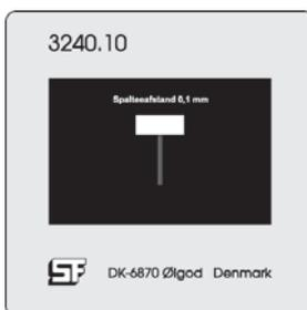
The frame with the double slit is oriented with the rectangular window upwards, making it possible at the same time to see the ruler through the window and the festoon lamp through the double slit.
