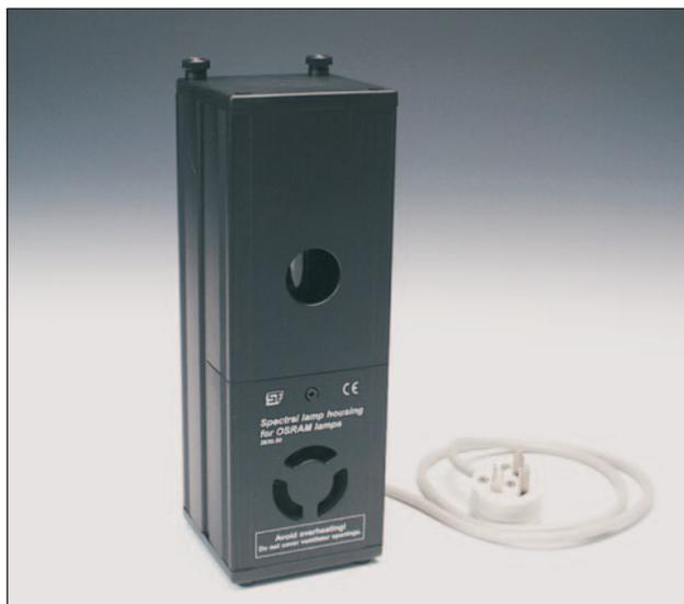
The spectral lamp housing is supplied with a three pole connecting cable and must only be connected to the mains supply via the control transformer 2840.50.
