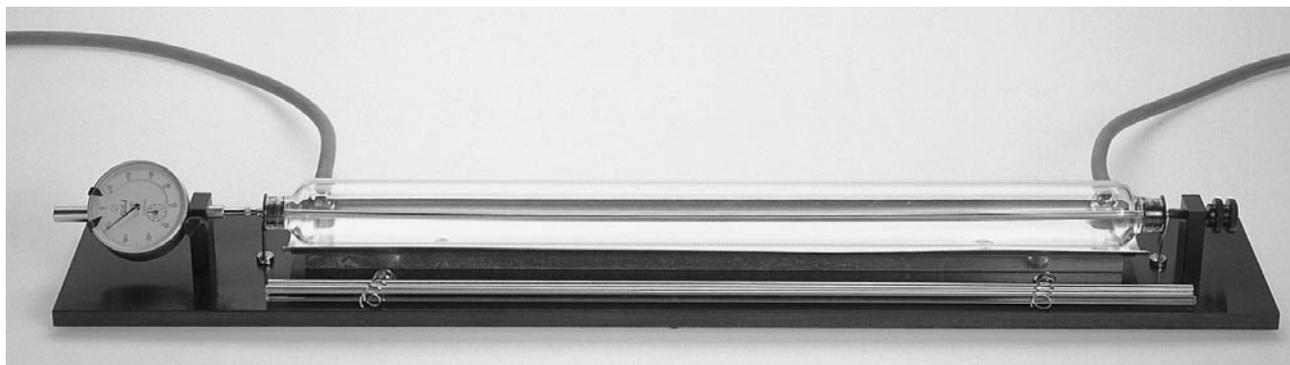
Apparatus for determination of the coefficient of linear expansion of iron, copper, aluminium and glass.
