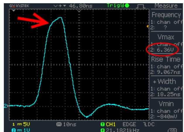
The image above shows a distorted pulse caused by too high amplitude.
