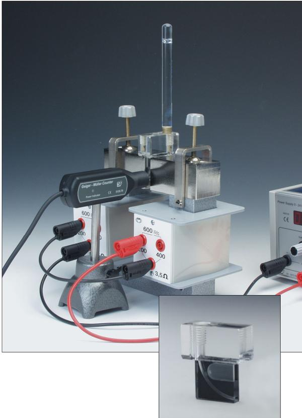
The equipment consists of a Perspex holder for a beta source with a quarter circular channel with a specific radius.
