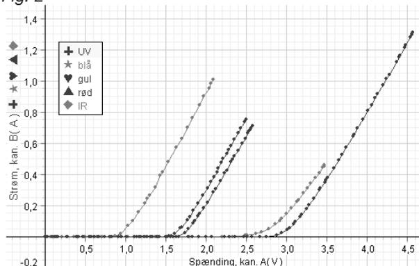
Characteristic curves for the various light emitting diodes recorded using the Pasco Science Workshop Interface and DataStudio software
