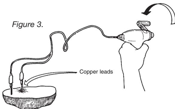
Turn the crank vigorously for about 30 seconds. Notice that a blue-green region will appear around one of the conductors but not around the other. This colouration only appears around the positive lead. The colouration is due to the formation of copper chloride which is created due to the electrolysis of salt (NaCl) which occurs naturally in the potato juice.
