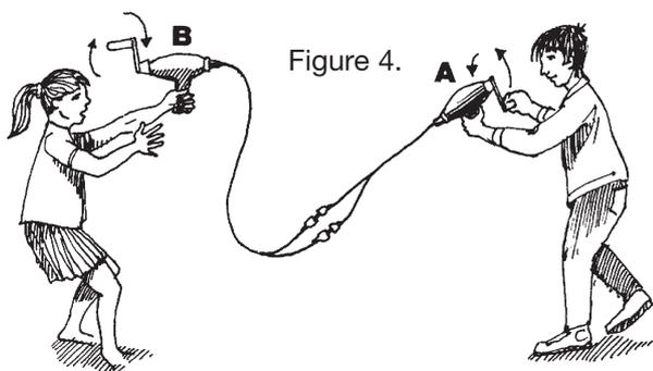
Call one generator A and the other B. When a student cranks generator A, the handle on B will begin to turn of its own accord to the surprise and delight of your students. Try turning the crank the other way. Change roles by cranking generator B and observing A.
