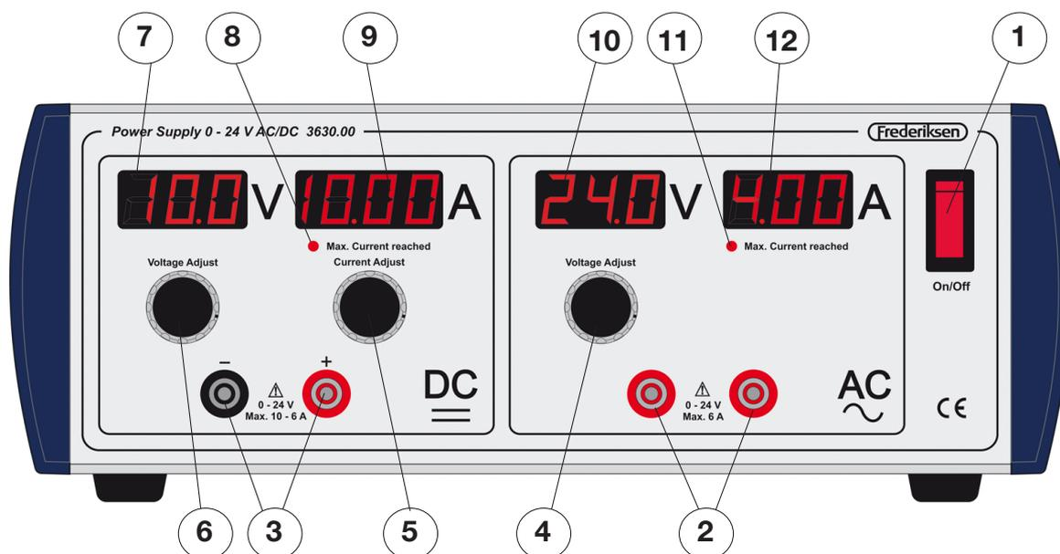
This power supply has been designed specifically for use in teaching physics, chemistry and other science subjects. The power supply can provide both direct current (DC) and alternating current (AC). The power supply can provide both types of electrical power at the same time, and they can be adjusted independently of one another. Separate displays are provided for DC and AC output.
