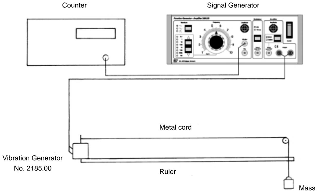
By repeating the experiment several times with different frequencies, it can be demonstrated that the velocity of propagation is independent of the frequency.
