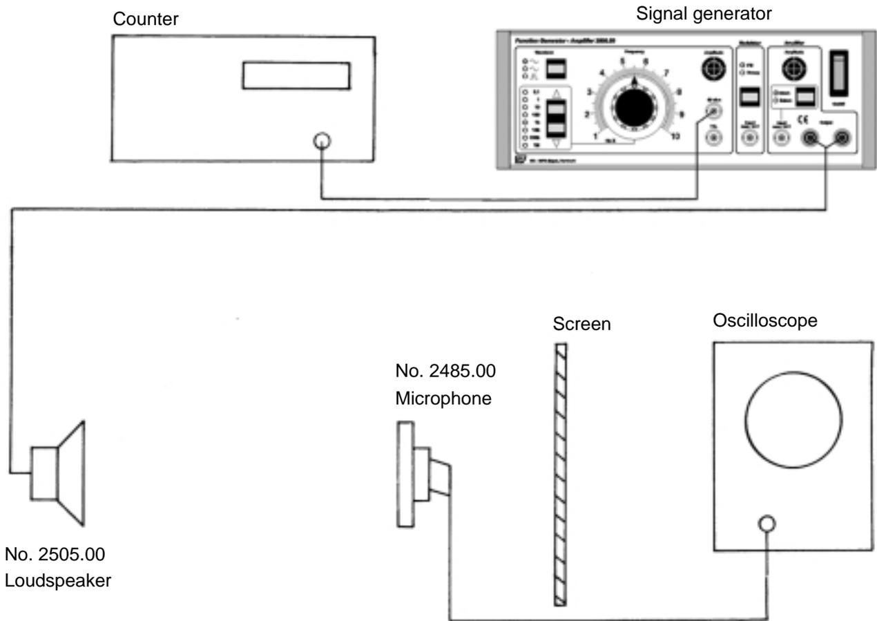
Variations in the sound intensity (variations in the height of the curves on the oscilloscope) may be observed by placing the microphone various places between the loudspeaker and the screen. Thus demonstrating that the sound is reflected by the screen and interferes with the forthcoming wave, resulting in standing waves. A graphic illustration of the results may also be drawn. The experiment may be extended by using screen of different materials e.g. mineral fibre, etc.
