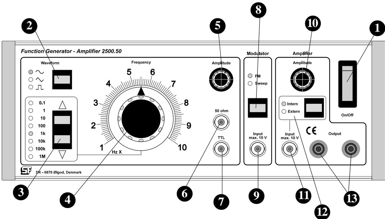
Pos. 5: Control button for adjusting the output signals' amplitude.
